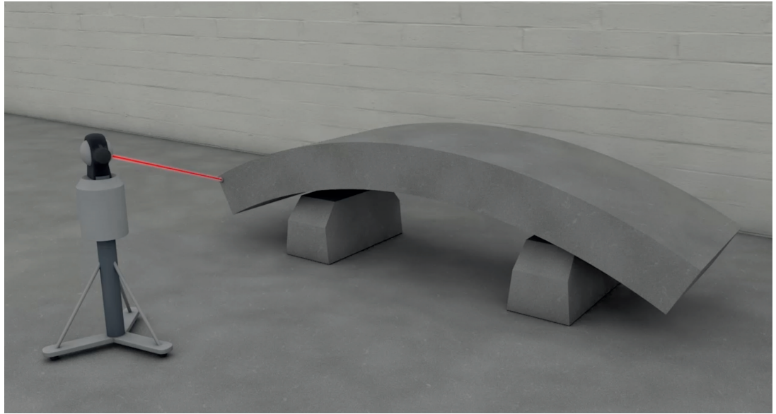
Right, figure 3: Alternative concept – virtual rings based only on digital measurement of segment production quality
