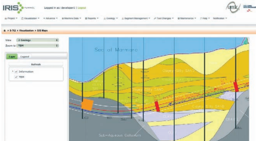
Above: Figure 4, IRIS tunnel data management system. Screenshot of the geology map visualization with the TBM position in real time
