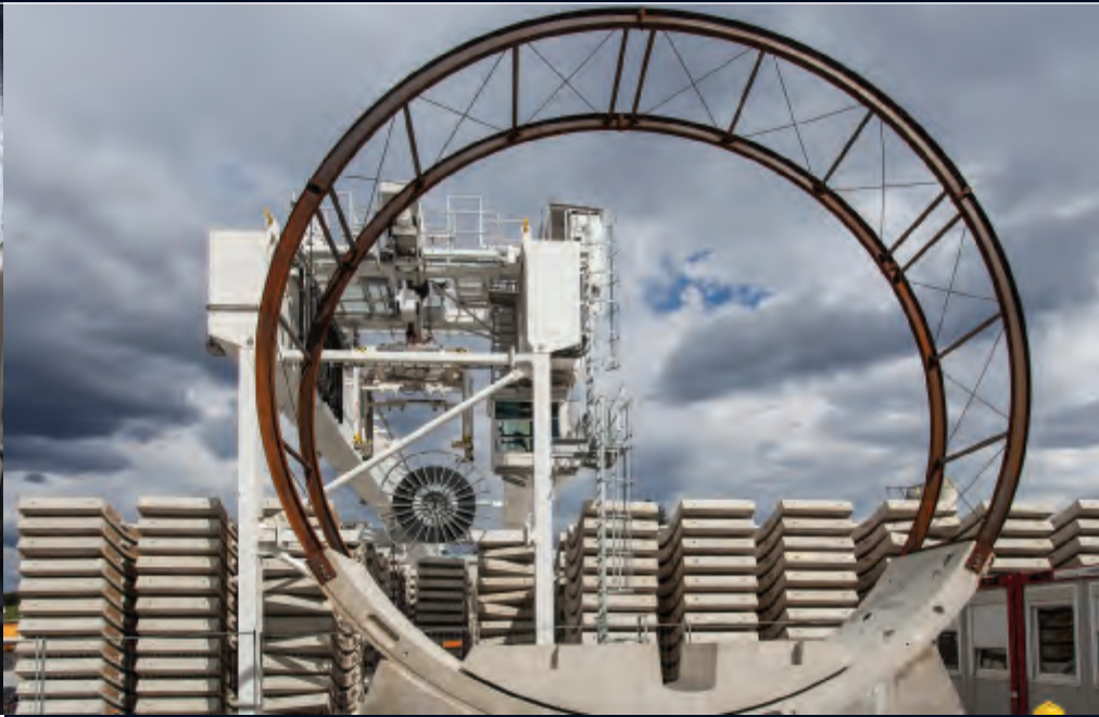
Above left: a partial Koralm Tunnel ring. Above right: barcoding of each individual segment
