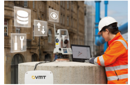
Deformation monitoring system
